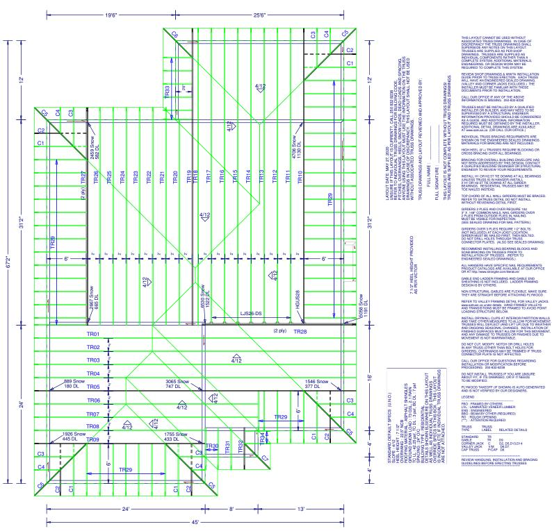
www.satruss.ca under details. HAND FRAMED VALLEYS AND TRANSISTIONS MUST BE FRAMED TO AVOID POINT LOADING STRUCTURE BELOW.
