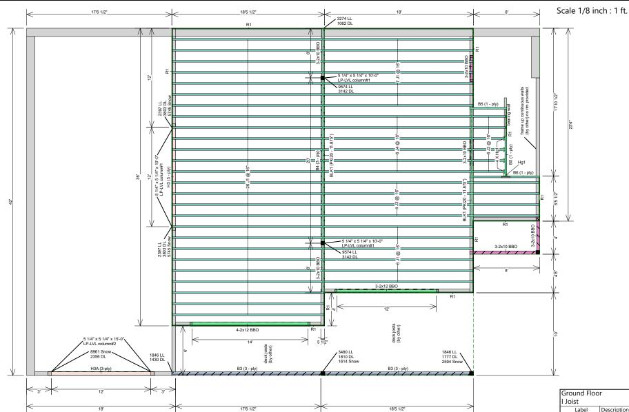
I-Joist and beam packages are rough cut / trim to exact length on site
