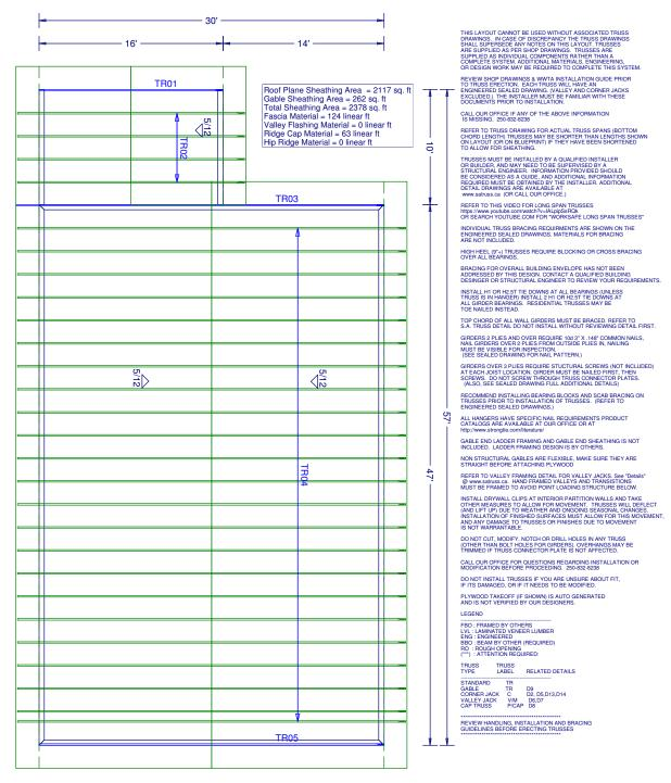
REFER TO TRUSS DRAWINGS FOR "ACTUAL" TRUSS SPECS STANDARD DEFAULT SPECS (U.N.O.) SLOPE : 5/12 HEEL: 7 1/2" GROUND SNOW LOAD: GSL 88 RAIN 2.1 DESIGN SNOW: 50.5psf TCDL: 5psf BCDL: 7psf SPACING: 24"oc BUILDING TYPE: Part 9 DETAILS SHOWN ELSEWHERE ON THIS LAYOUT AS WELL AS INDIVIDUAL TRUSS DRAWINGS OVERRIDE SPECS IN THIS BOX. THIS LAYOUT IS INCOMPLETE IF INDIVIDUAL TRUSS DRAWINGS ARE NOT ATTACHED.
